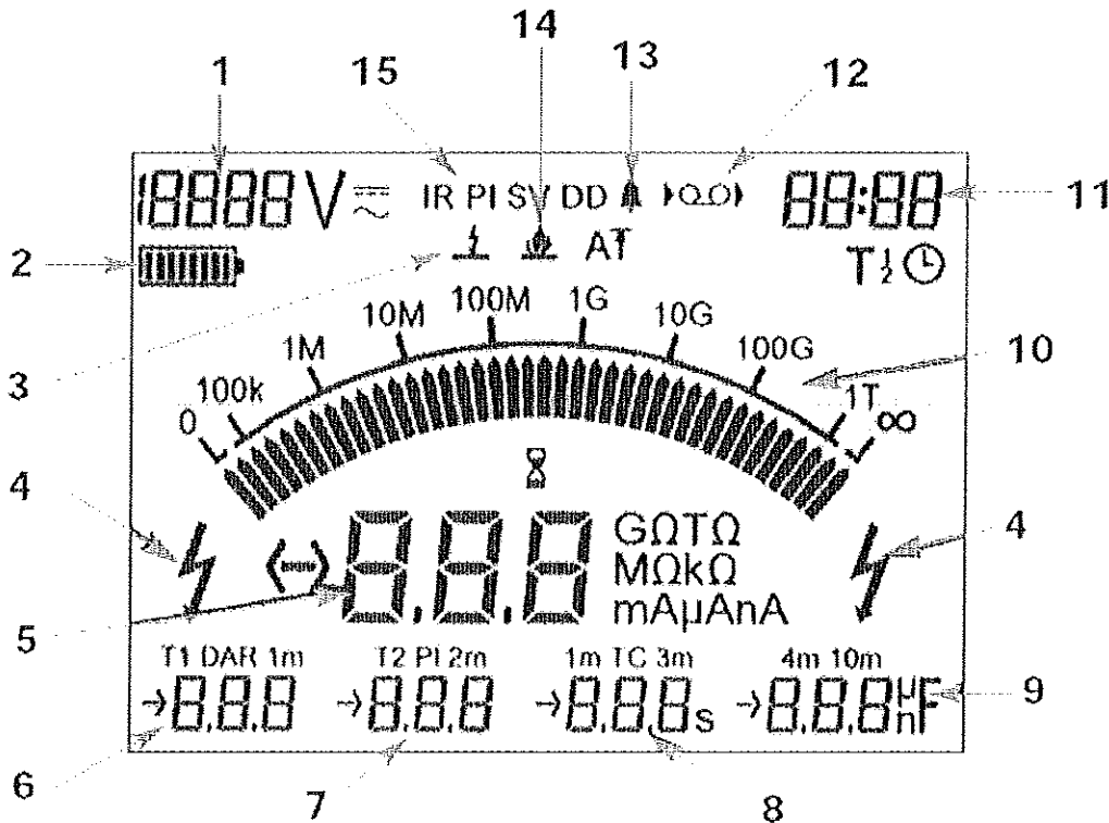
Fig. 2: Insulation resistance digital display.
